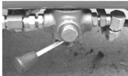
Rotary valve lever left position |
